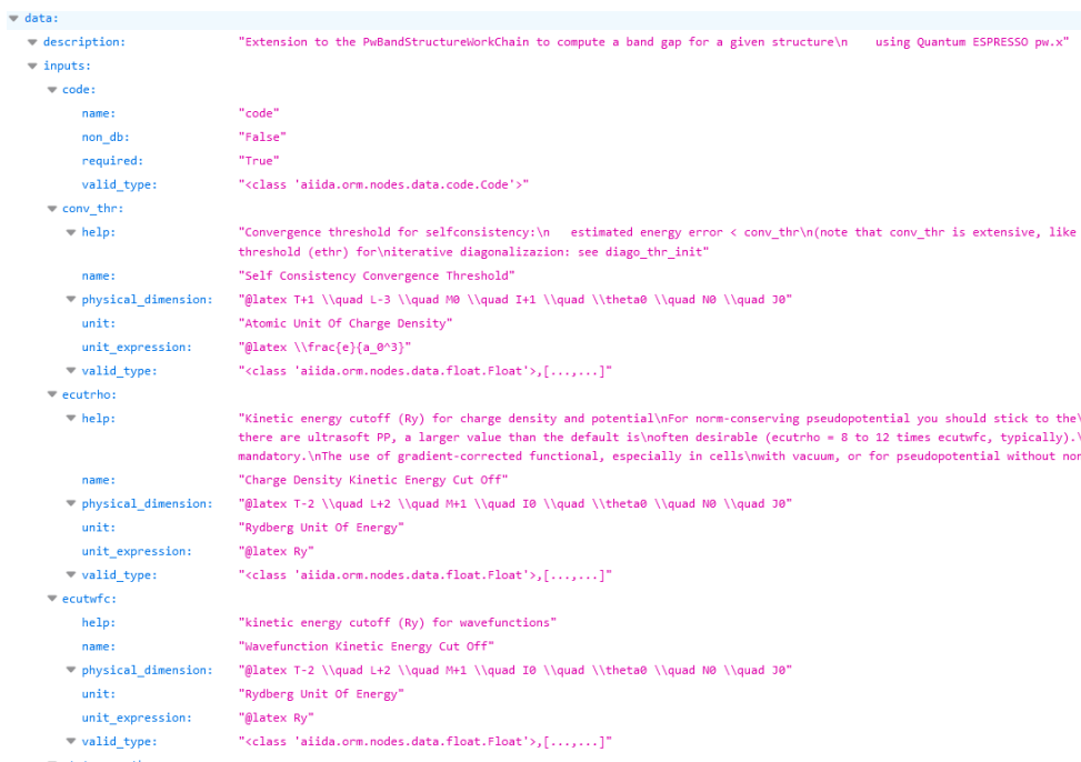
Figure 4: Example response to a query for http://localhost:8000/api/v4/intersect/properties/band_gap.pw/inputs/intermediate with respective parameters like the self-consistency threshold for the simulation convergence, cut off energy for the charge density, etc.
