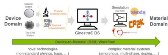
Figure 1. Schematic representation of the proposed methodology. (left to right) Electrical data measured on material blankets/test chips are given as input to the Ginestra® simulation platform.
